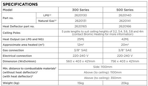
'Must only be installed by a licensed technician. Must complete "Pre-Installation Checklist" before installing <sup>2</sup>The temperature will not exceed 65°C above the ambient temperature at specified distances. Please consult material manufacturer for temperature ratings and suitability. Bromic Heating takes no responsibility for material compliance.
