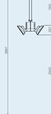
CEILING POLE CLEARANCE WITH HEAT DEFLECTOR
