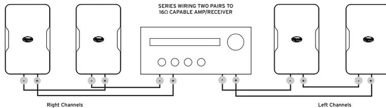
If your amp/receiver cannot drive a two-pair, 4 Ohm load above, connect both pairs of CP-6's to the single set of speaker terminals in series as shown. This will lower the volume sent to all speakers.
