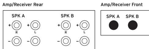
If your amp/receiver has separate connections for two speaker pairs, connect the two pairs of CP-6's to the two speaker terminal sets. Depending on your amp/receiver, either both pairs, or just one pair, will play at the same time.
