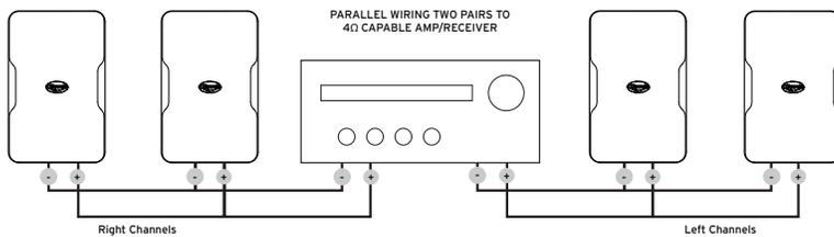
If your amp/receiver does not have separate connections for two speaker pairs, connect CP-6's to the single set of speaker terminals in parallel as shown. Your amp/receiver must be rated to 4 Ohms to make this connection.
